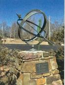
"The proposed sundial will consist of several hoops and rings, marked by various symbols and pierced by an arrow. The sundial will be made of cast bronze and will measure 30" high and 24" wide. The rings and hoops will be supported by a flat bronze base with zodiac symbols. The flat bronze base will anchor to the stone.
